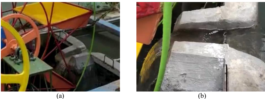
Fig. 2. Modified trapezoidal sharp crested overflow front view (a), and side view (b)
