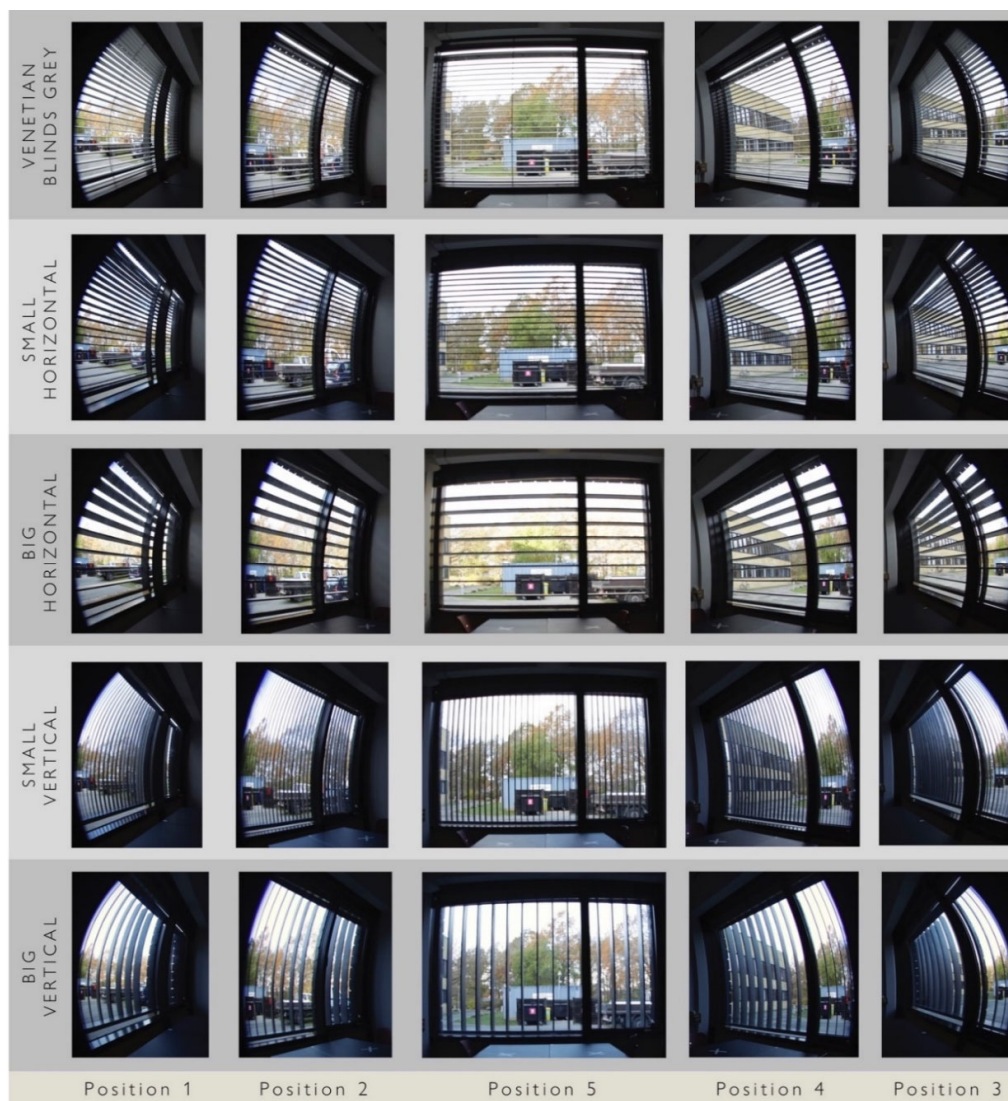
Figure 3: An overview of the different solar shading conditions seen from each subject position in one of the rooms.
