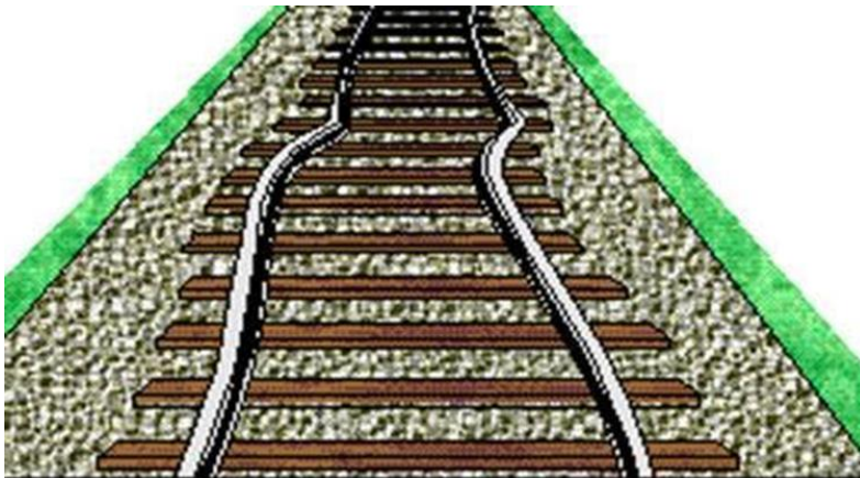
Fig. 2. Railroad track ejection
