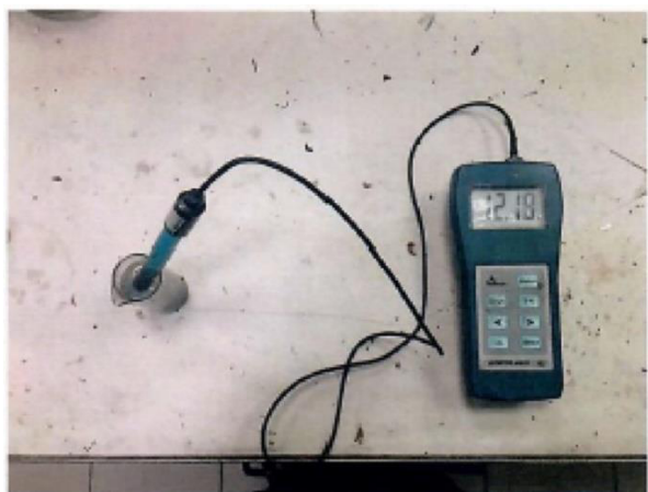
Fig. 10. pH measurements of foam concrete.
