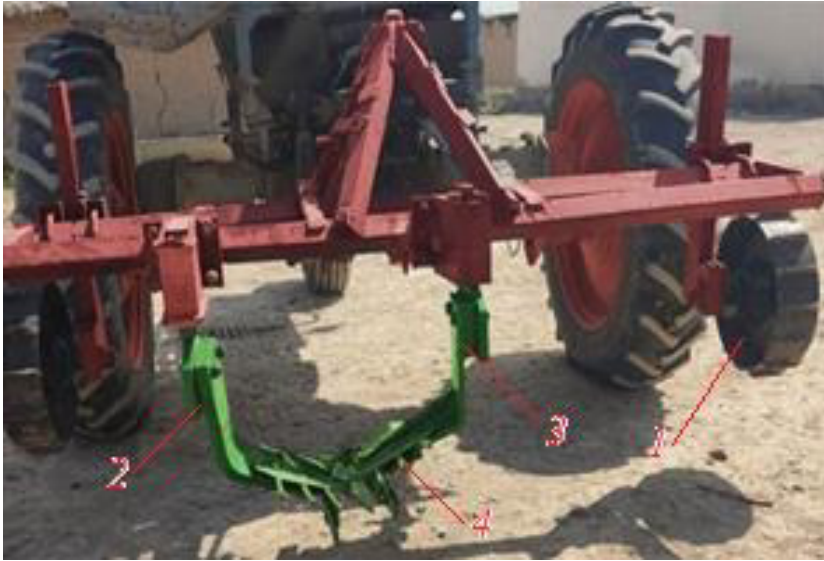
Fig. 2. General view of the potato digger with working bodies of the "paraplaw" type
