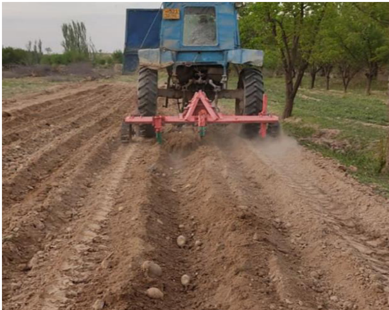
Fig. 3. The process of work of the potato digger with working bodies of the "paraplaw" type
