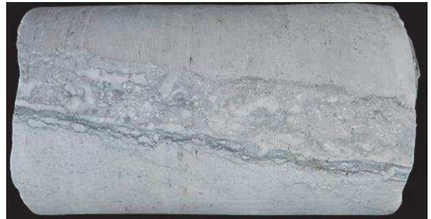
**Fig. 12.** Side view in white light photo of carbonate RSWC (wellbore end on the right side).
