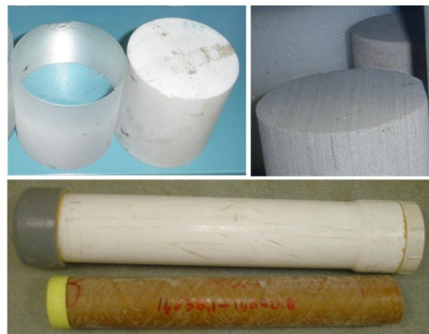
Fig. 4. Calibration ‘standards’ - quartz, Macor, Berea and a representative cleaned sandstone (top). Blank PVC core box and fiberglass core sleeve (bottom).
