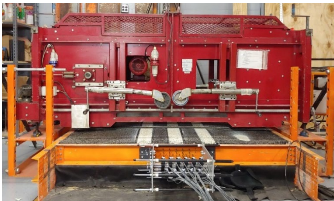
Fig. 14. Model Mobile Load Simulator (MMLS) trafficking a pavement test section.
