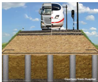
(a) schematic view Fig. 8. Geosynthetics encased stone column technique.
