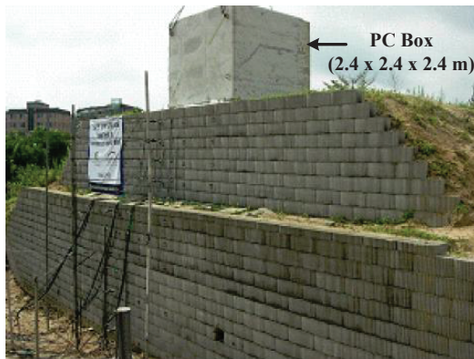
(a) test wall configuration Fig. 7. Full-scale test wall configuration and results [9].
