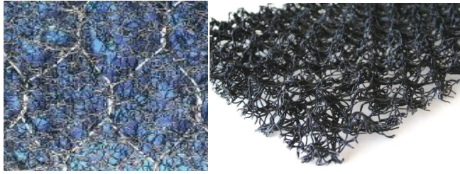
Fig. 3. Reinforced geomats with steel wire mesh (left) and polymeric geogrid (right)
