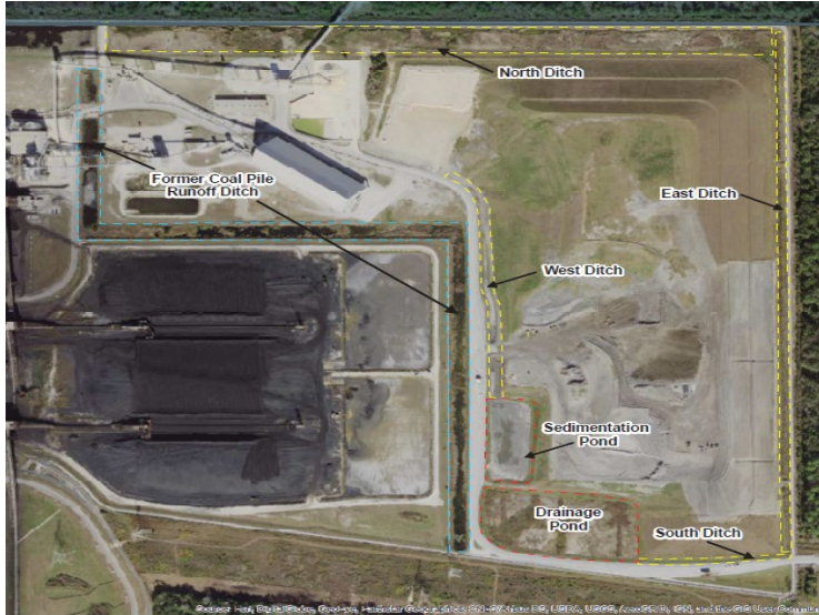
Fig. 1. Existing CCR landfill stormwater management system.
