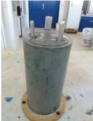
Fig.4. Insertion of three vertical drains
