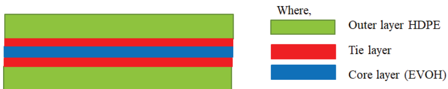
Figure 4: Schematical representation of HDPE/EVOH structure for barrier geomembrane
