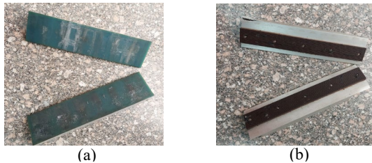
Fig. 3. Uniaxial tests' clamps: (a) Plastic-lined clamps; (b) Serrated steel-lined clamps.
