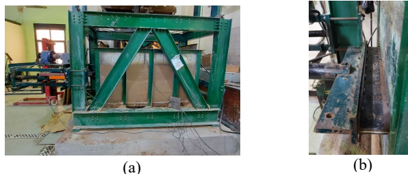
Fig. 4. Pull-out test setup: (a) Apparatus; (b) Clamp.
