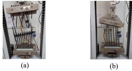
Fig. 5. Uniaxial specimen failure in tensile tests: (a) GG1 with serrated steel-lined clamps; (b) GG2 with plastic-lined clamps.
