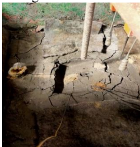
Fig. 6. Clay Failure Shape
