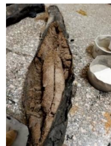
Fig. 8. Slag – Cement Dust Soil Mixture After the Test
