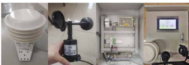
Figure 8. Equipment of building networking monitoring system
