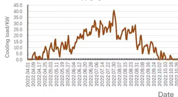
Figure 6. Daily Cooling Load Curve of Enclosure Wall under Closed Cold Aisle of Sever Room
