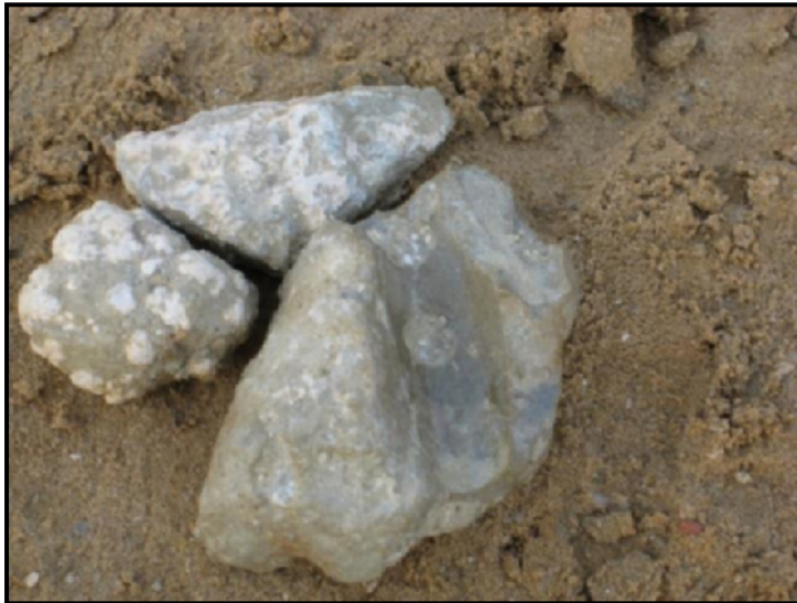
Fig. 6. Thin (thickness 20 cm) stone crust. Sample taken from the depth of 19 m.
