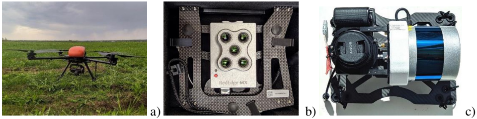
Fig. 2. Geoscan 401 with Sony RX1R2 camera (a), RedEdge-MX multispectral camera (b), Lidar AGM MS-1 (c). Source: Compiled by authors.
