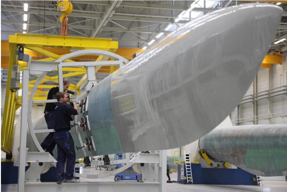
Fig. 1. Vacuum infusion production of wind blades [7].
