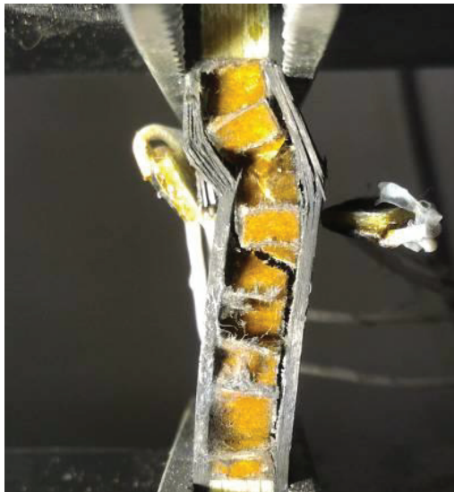
Fig. 5. Failure pattern of specimen ( l = 35 mm, h = 5 mm).
