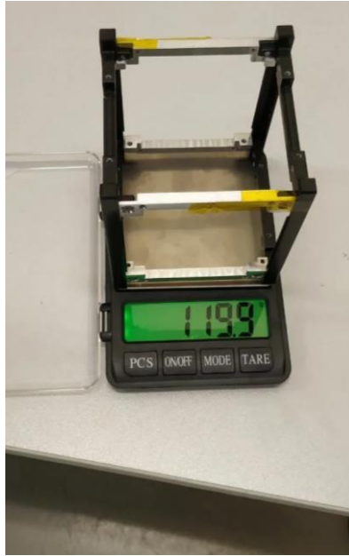
Fig. 10. Masst of the aluminium construction.
