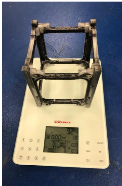
Fig. 9. Mass of the carbon fiber construction.
