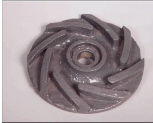
Fig. 9. Reconditioning of pump impeller.
