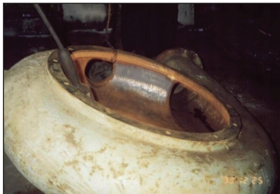
Fig. 7. Reconditioning of rotor.
