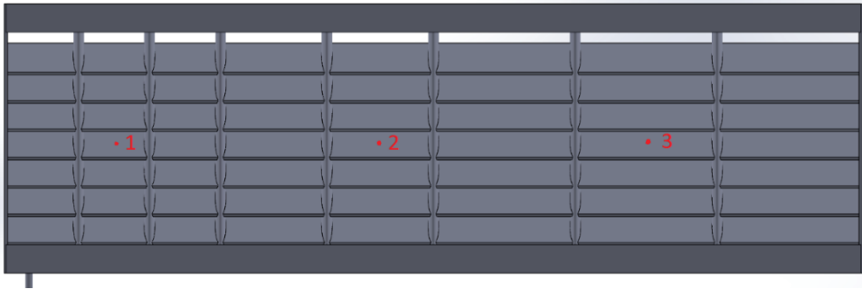
Fig. 8. Points for taking temperature values (1 - small section, 2 - middle section, 3 - large section).
