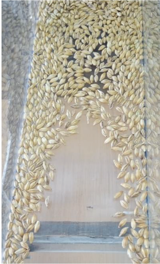
Fig. 6. Grain displacement towards the periphery on an inclined vibrating surface. Source: [Author's study].
