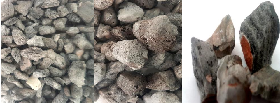
Fig. 1. Grains of expanded obsidian of different size and average density.
