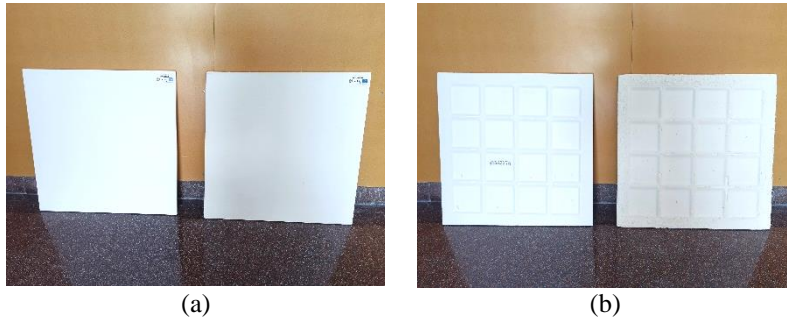
Fig. 2. Standard and PU-gypsum precast.
