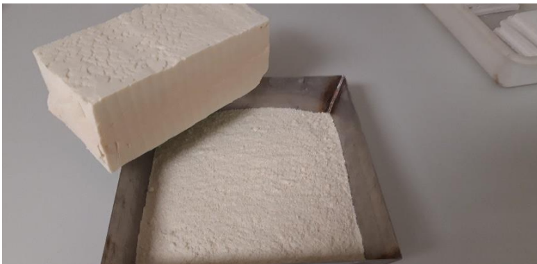
Fig. 1. Polyurethane foam waste. Before and after crushing
