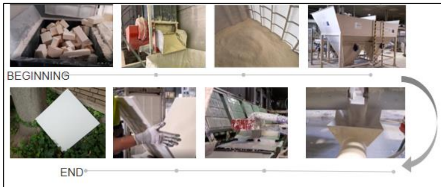
Fig. 4. Industrial manufacturing process of PU-Gypsum ceiling tile.
