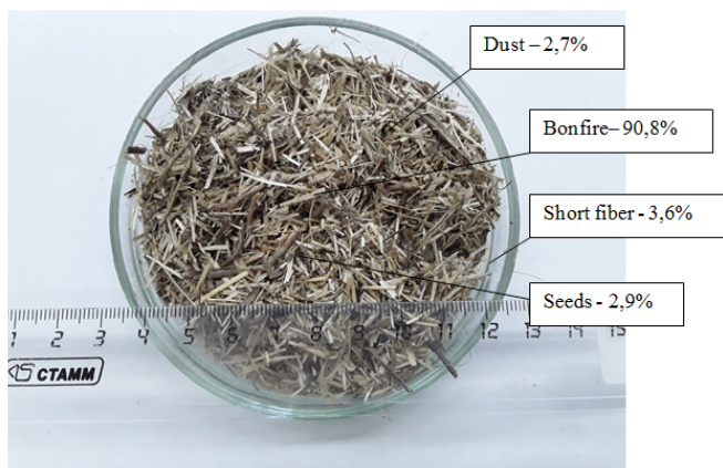
Fig. 2. Composition of the bonfire mixture: dust - 2.7%, shives – 90.8%, meek fiber - 3.6%, seeds - 2.9% ("Compiled by the authors").
