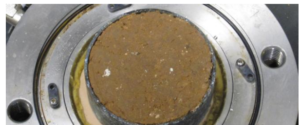
Fig. 18a. Net normal vertical stress 25 kPa; PI=27, compacted specimen, dried to suction of 400 kPa [73]
