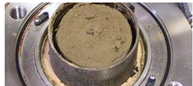
Fig. 18b. PI=42 specimen dried from slurry to 400 kPa suction under total vertical stress of 3 kPa [73]
