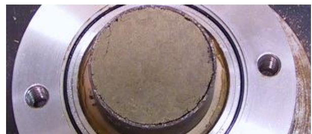
Fig. 18c. PI=42 compacted specimen dried from s=0 to 400 kPa suction under total vertical stress of 3 kPa [73]
