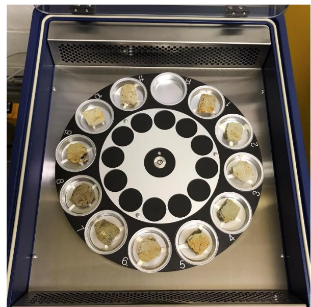
Fig. 2. Sample tray inserted inside the sealed chamber.
