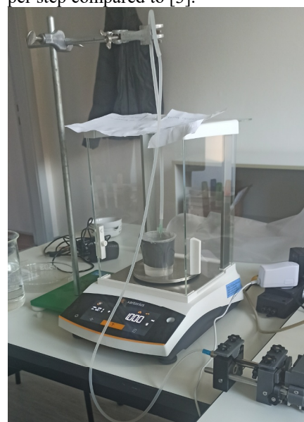
Fig. 1. Calibration set-up for determining the inner syringe diameter using weight-controlled pumping tests.
