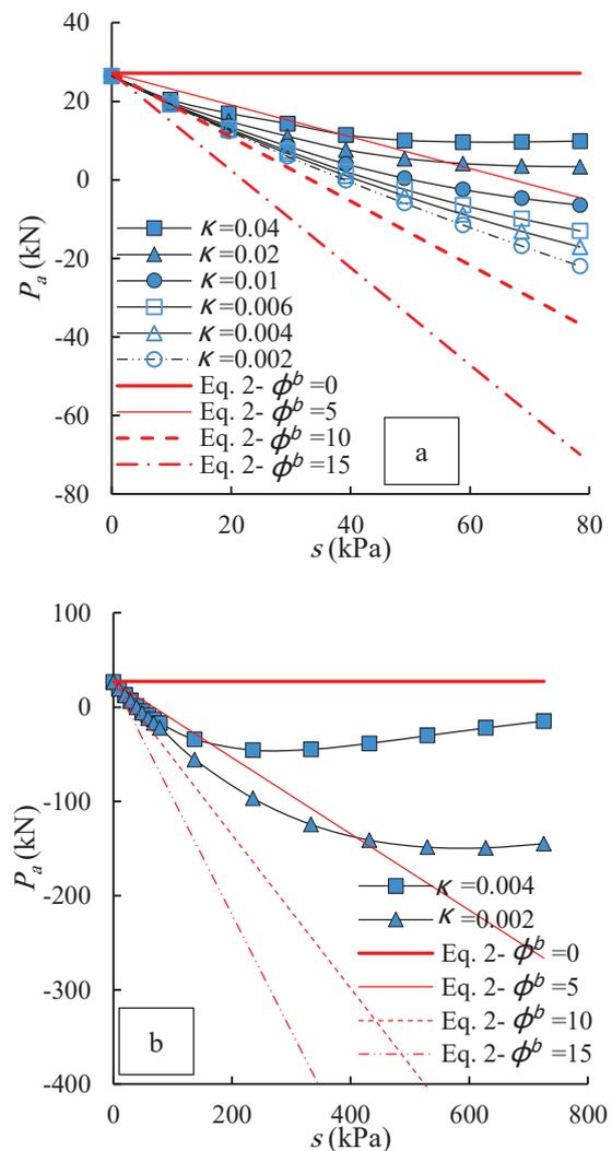
Fig. 6. The effect of: (a) soil types and (b) the hydraulic and/or mechanical hysteresis on the active thrust,  $P_a$ .
