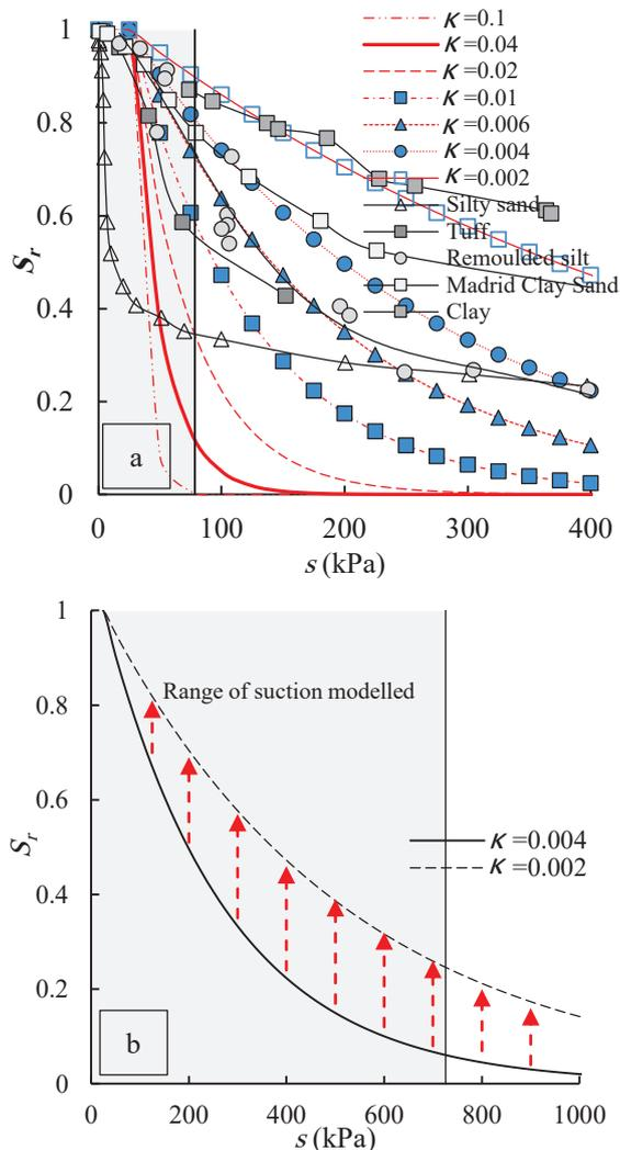
**Fig. 3.** (a) WRCs for various soils fitted using Eq. 1 at various  $\kappa$  values and plotted against available SWRCs and (b) SWRC of two different soils considering hydraulic and mechanical hysteresis.
