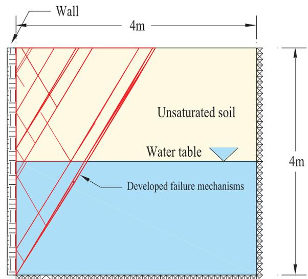
**Fig. 4.** Problem geometry for the modelled retaining wall.
