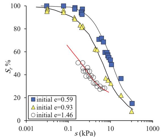
**Fig. 2.** Mechanical hysteresis of a soil, after [11].
