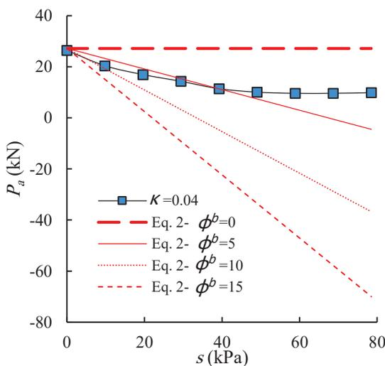
Fig. 5. Validation of the UNSAT-DLO approach against Eq. 2.
