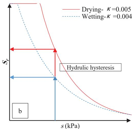
**Fig. 1.** (a) WRCs for various soils available from the literature and (b) Hydraulic hysteresis of the SWRC.
