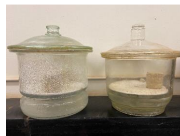
Figure 1 Vapor equilibrium chambers used to impose the total suction on the soil samples along the wetting and drying paths.
