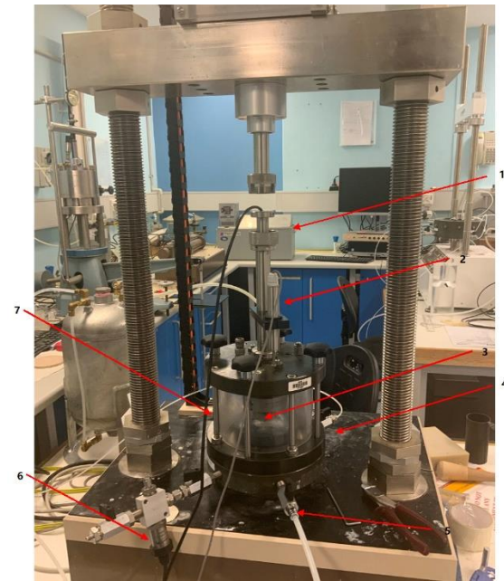
Fig. 3. Dynamic CRS equipment used in this study. Parts shown in the photo are: 1) Loading ram; 2) Axial displacement transducer; 3) Load cell; 4) Back pressure valve; 5) Cell pressure valve; 6) Pore water pressure transducer; 7) CRS cell.
