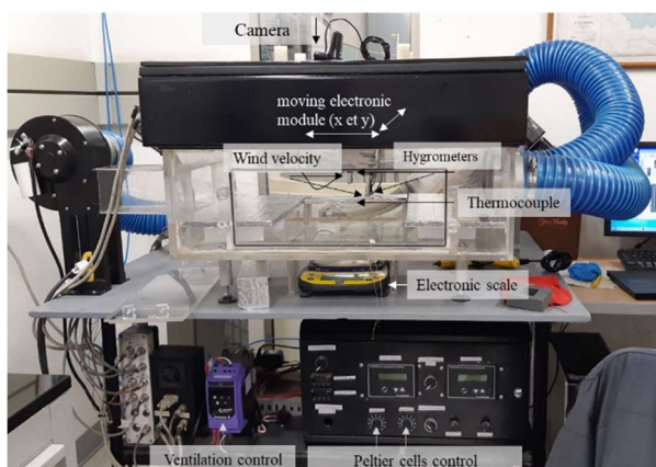
Fig. 1. General view of the climatic chamber.
