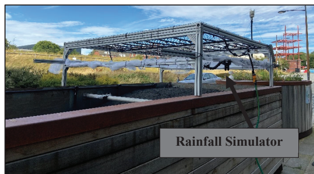
Fig. 2. Photograph illustrating the placement of the rainfall simulator on top of the lysimeter to apply storm events.
