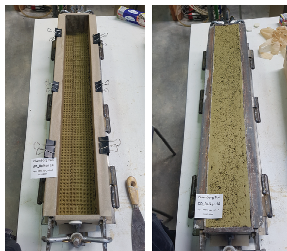
Fig. 3. First and last layer of the installation process of GD.
