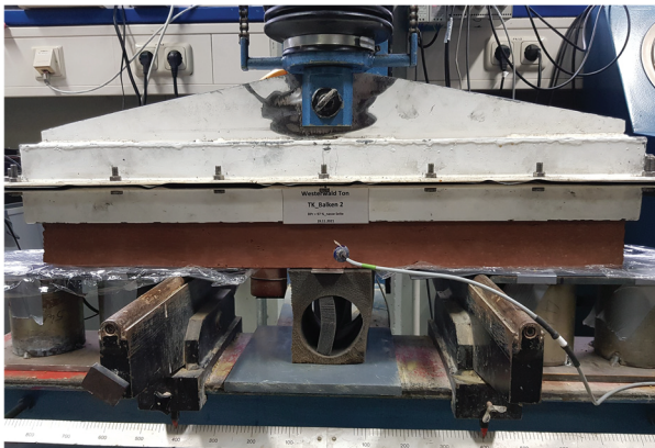
Fig. 5. TK clay beam with one tensiometer before testing.
