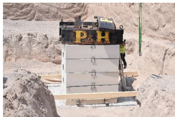
Fig. 9. View of the elements used for the application of the test load.
