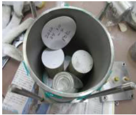
Fig. 2. Specimens with a salt solution in the steel mold.
