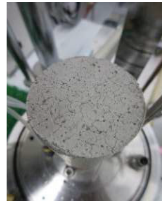
Fig. 6. Cracks under free deformations and heating.
