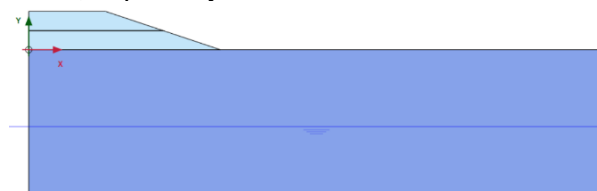
Fig. 10. Embankment geometry in PLAXIS 2D.
