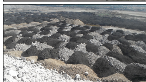
Fig. 1. Examples of tailings disposal solutions. (a): tailings disposed in a cell; (b): desiccated tailings, 8 months after disposal in a cell (from [2]). (c) co-disposal of mixed plant reject (MPR) from a tiphead (from [2]); (d): paddock tipping amongst waste rock (from [3]).
