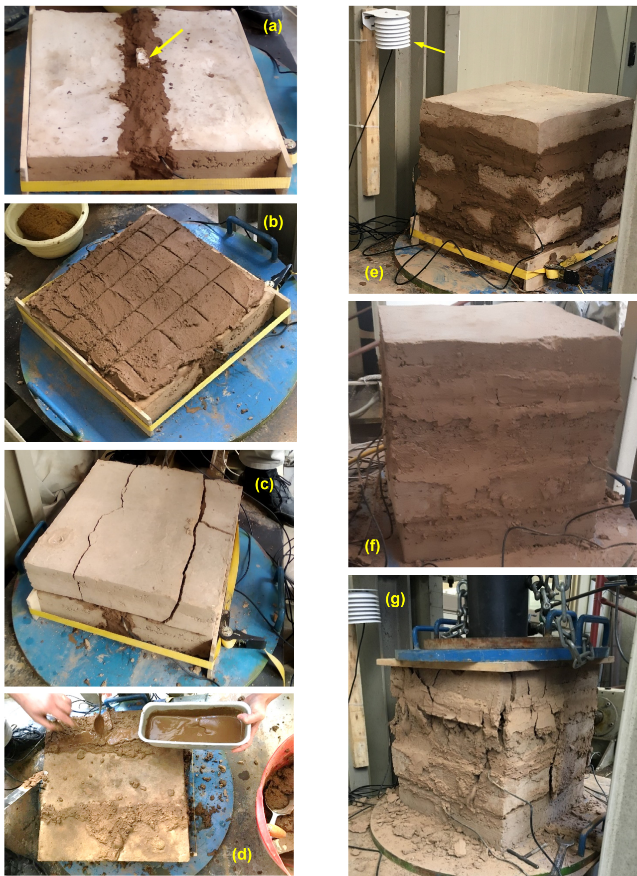
Fig. 7. a) Bottom row of half-size mudbricks for the 0% content of dry grass (arrow indicating TEROS12 sensor installed in fresh soil mixture used as mortar), b) first horizontal layer just applied, c) first whole mudbrick with sensors heavily cracked, d) finer fraction slurry prepared to fill cracks, e) small mudbrick wall just built (arrow indicating relative humidity sensor), f) the same wall after drying to constant conditions, and g) the same wall during loading close to peak strength (severe cracking already developed).
