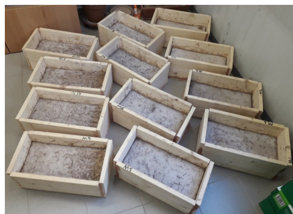
Fig. 2. a) Whole mudbricks positioned in atmospheric conditions for drying (arrows denoting mudbricks with sensors installed -pointing to sensor cables coming out of the samples), and b) half-size mudbricks.
