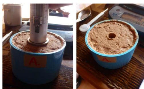
Fig.9 Yamanaka test for filled sand with samples of different water content by drying step
