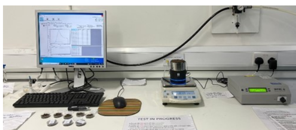
Fig. 2. Control PC (left), HYPROP (middle), WP4C (right).
