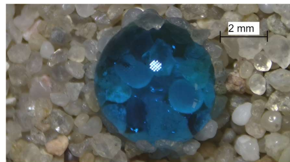
Fig. 1. Drop of dyed water resting on the surface of a hydrophobic sand sample.
