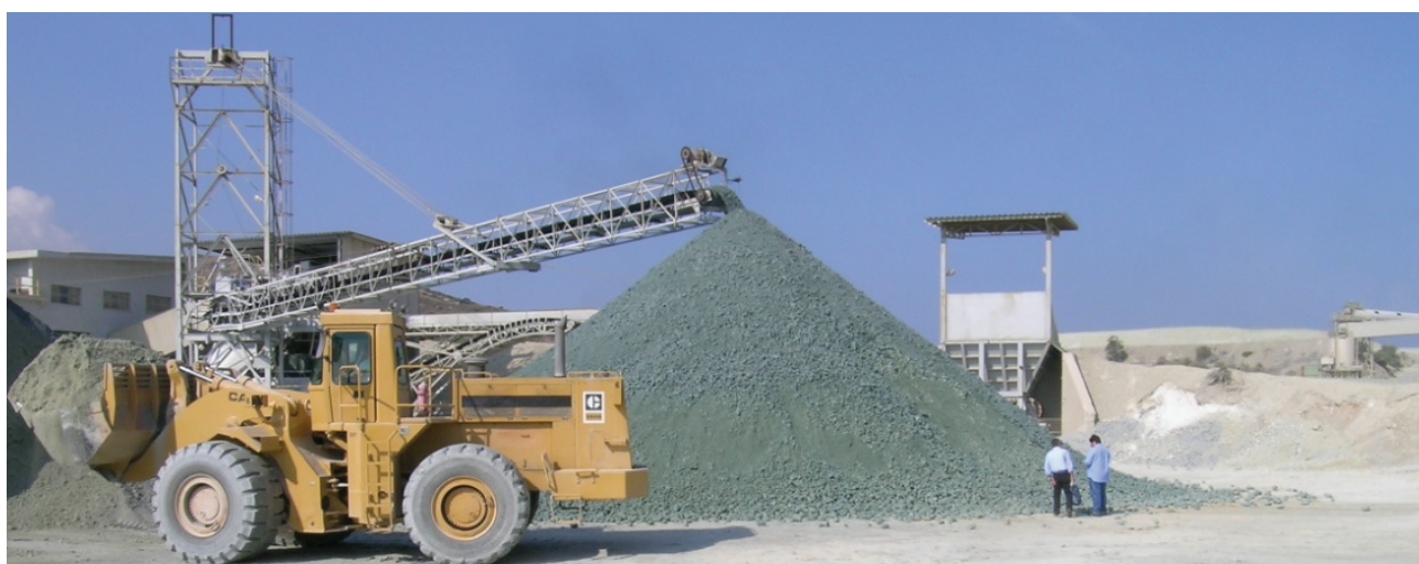
Fig. 16. The soda-activated bentonite is ready to enter the processing plant for drying.
