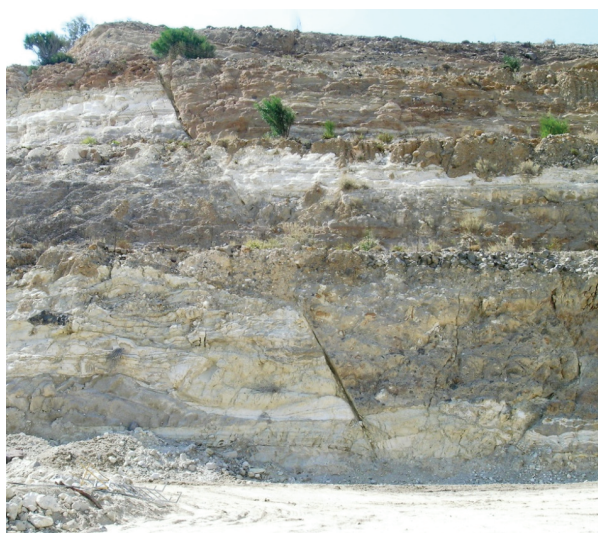
Fig. 7. A quarry face at the Xylokeratia quarry of pozzolanas. Note the mixture of brown lapilli and grey fine-grained tuffs, with the white biogenic silica rich beds (diatomite). Faults are common in all quarries and outcrops across the island.
