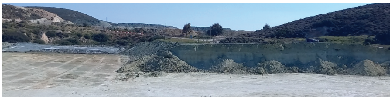
Fig. 17. Yard which hosts soda activated bentonite in successive beds of different qualities. The vertical extraction of the beds is beneficial allowing total homogenization of the bentonite to be achieved.
