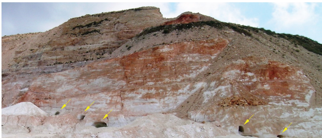
Fig. 6. The Kastriani kaolin S&B quarry in the late 90's. The old underground works can be seen (arrows). The specific quarry now accepts the perlite fines of IMERYs SA, as backfill.
