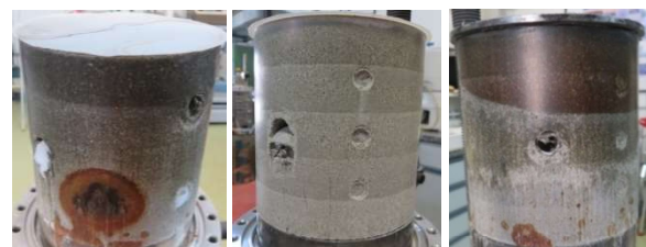
Fig. 5. Appearance of the bentonite blocks of cells C1, C1h and C1h_2 (from left to right) once extracted (heater surface at the bottom, the five compaction layers are visible, as well as corrosion stains).
