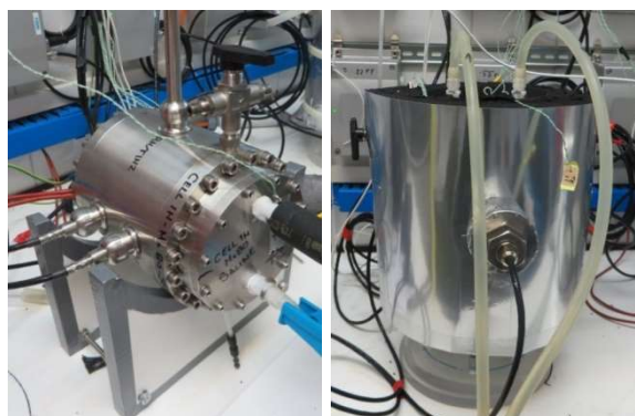
Fig. 1. Appearance of cells C1h and C1 before and after being covered by the insulating material.
