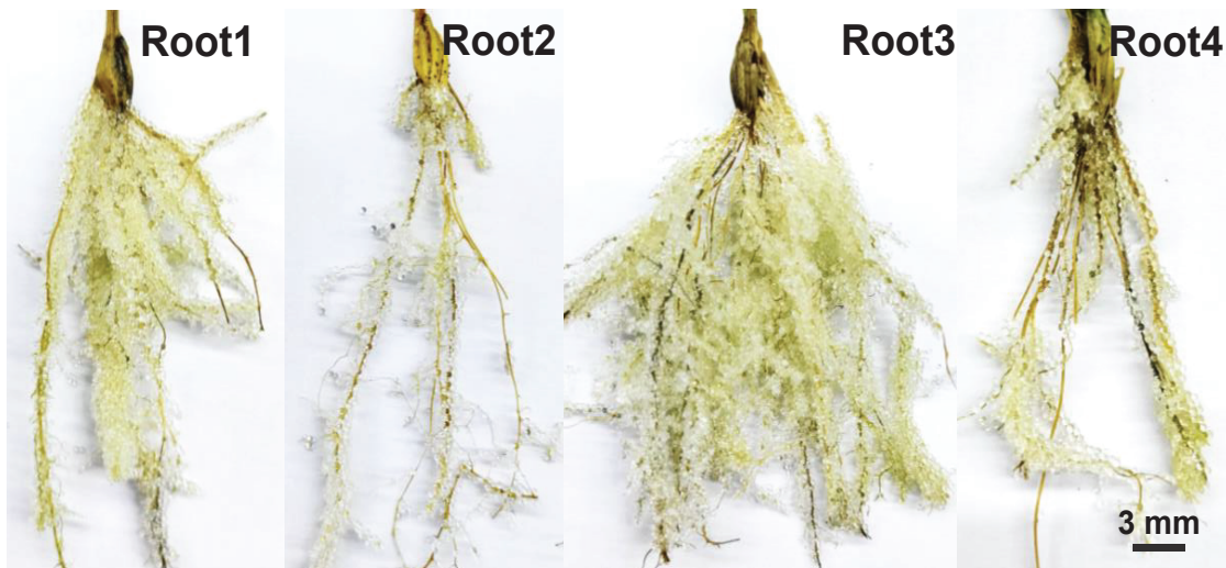
Fig. 17. Images of the four individual root systems exhumed from the planted sample Bar4 after testing.
